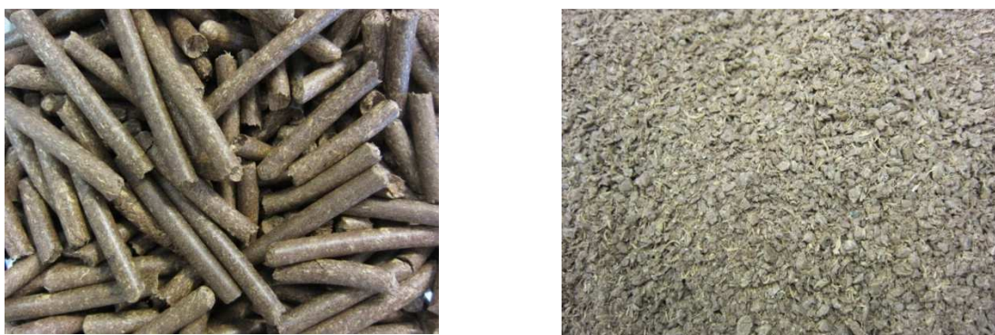
Figure 7: Sorghum pellets (left) with the grinded pellets (right).
