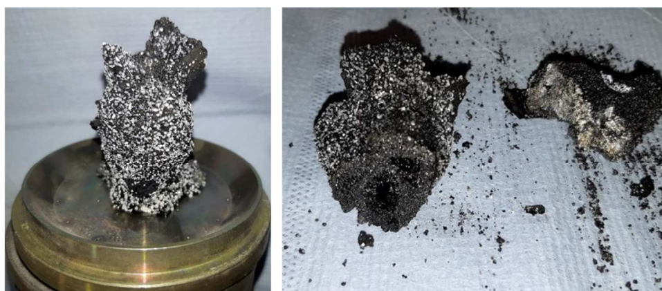
Figure 38. Unconverted solidified biooil accumulated during the gasification test #3.
