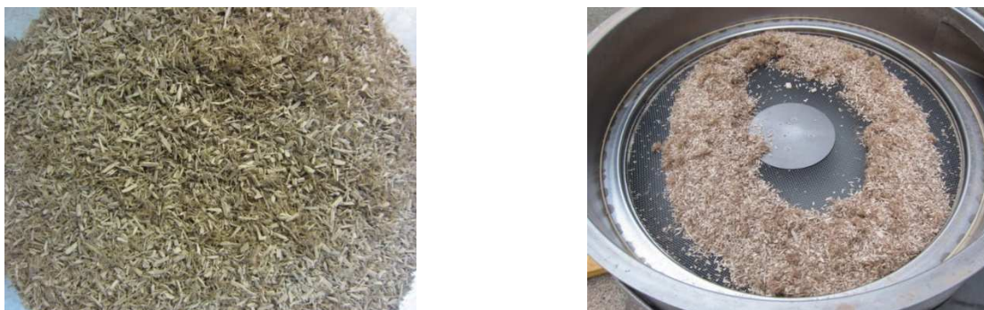
Figure 6: Eucalyptus <2mm sieve fraction (left) with the residue (right).
