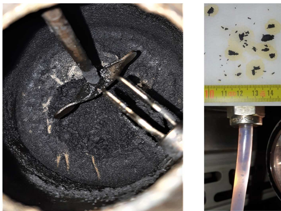
Figure 31. Slurry fouling and char clusters developed in the feeding system.
